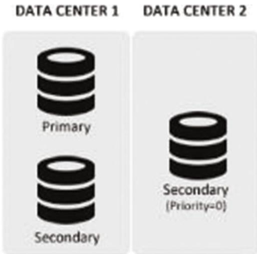
Figure 7-8. Members replica set with primary, secondary, and a priority 0 member distributed across the data center
