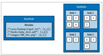
*Figure 1-1. An HDFS cluster with a replication factor of two; the NameNode contains the mapping of files to blocks, and the DataNodes store the blocks and their replicas*
