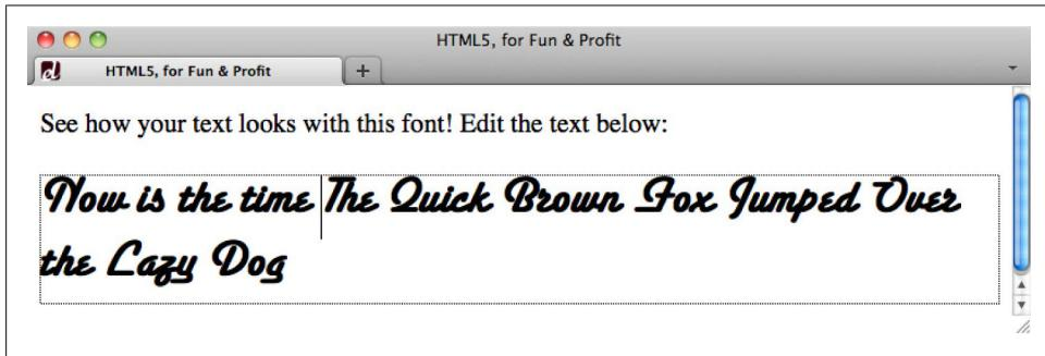
Figure 1-11. Once focus is set on an element assigned `contenteditable`, Firefox 5.0 displays a gray dotted line around it, indicating the area that can be edited
