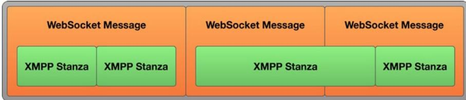
**Figure 4-5.** Stanza-to-message alignment (XMPP over WebSocket subprotocol draft proposal)
