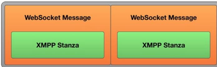
**Figure 4-6.** No stanza-to-message alignment (WebSocket to TCP proxy)
