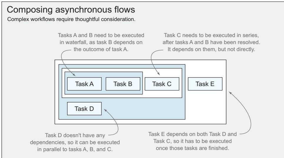
**Figure 6.4** Dissection of a complex asynchronous flow. Hint: always group tasks, in your brain, according to their requirements.
