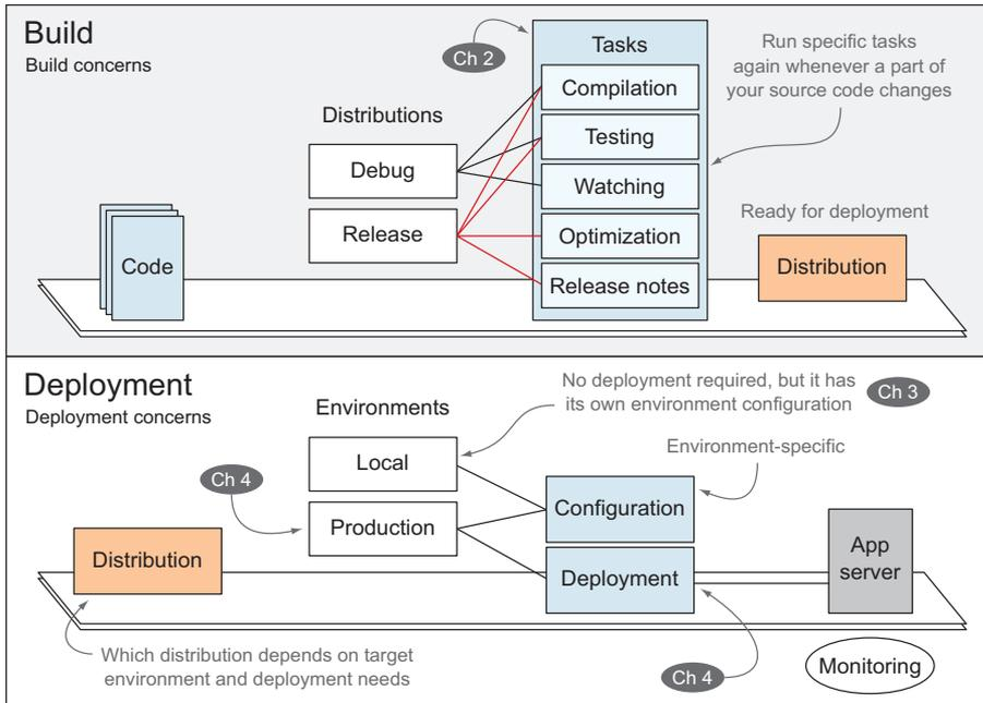
**Figure 1.2 High-level view of the processes in Build First: Build and Deployment**
