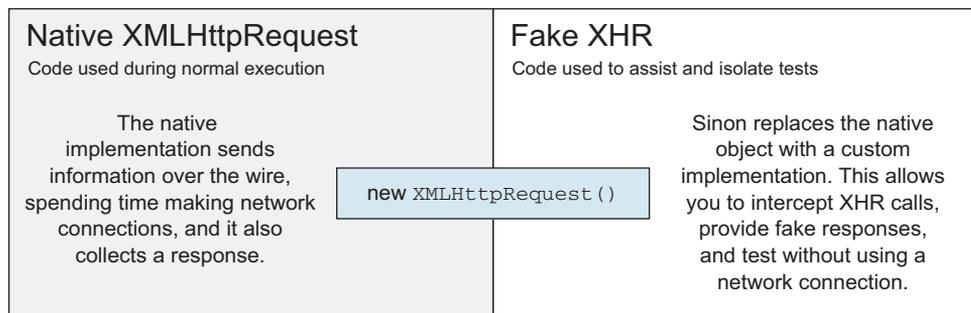
**Figure 8.3** Native XMLHttpRequest compared with fake XHR mocks during tests
