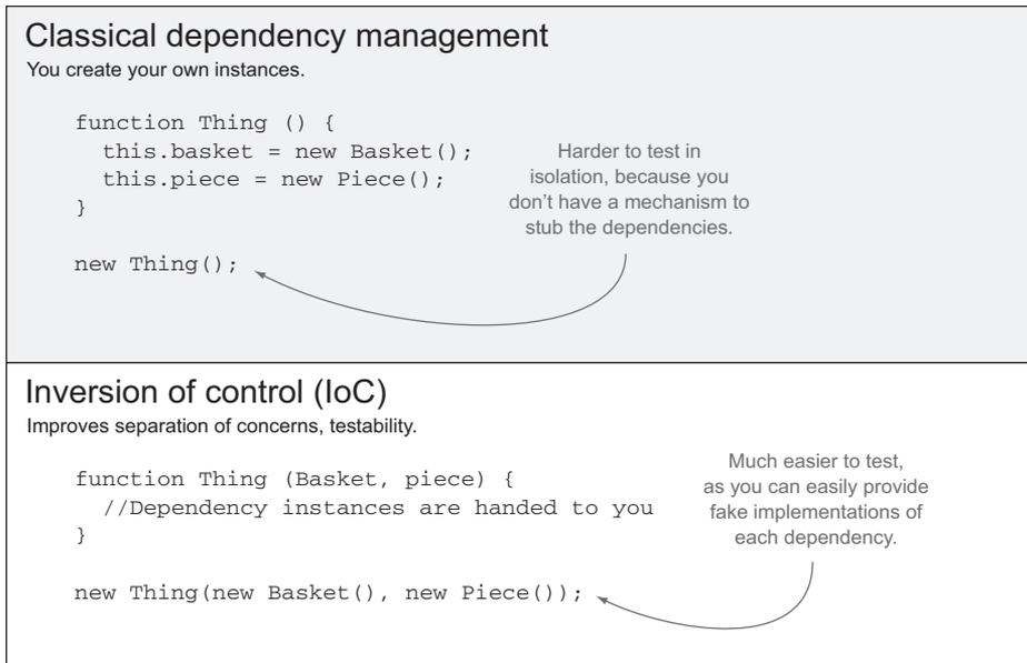
**Figure 5.3** Classical dependencies compared with using IoC to improve testability
