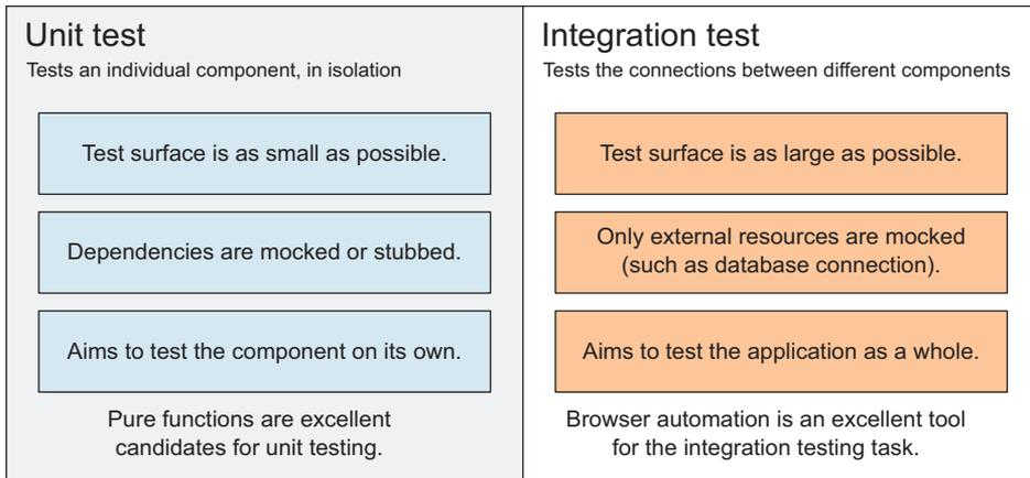
**Figure 8.1** Differences between unit and integration testing strategies. Note that a combination of the two should be used. Unit tests and integration tests are not exclusive. Pure functions are discussed in section 8.1.15.
