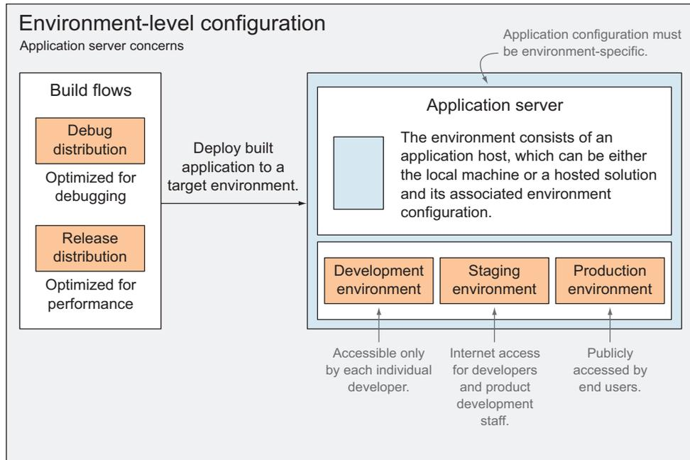
**Figure 3.2 Environment-level configuration—environments, configuration, and distributions, coming together in an application. Environment configuration consists of secret credentials and any other configuration that might change across environments.**
