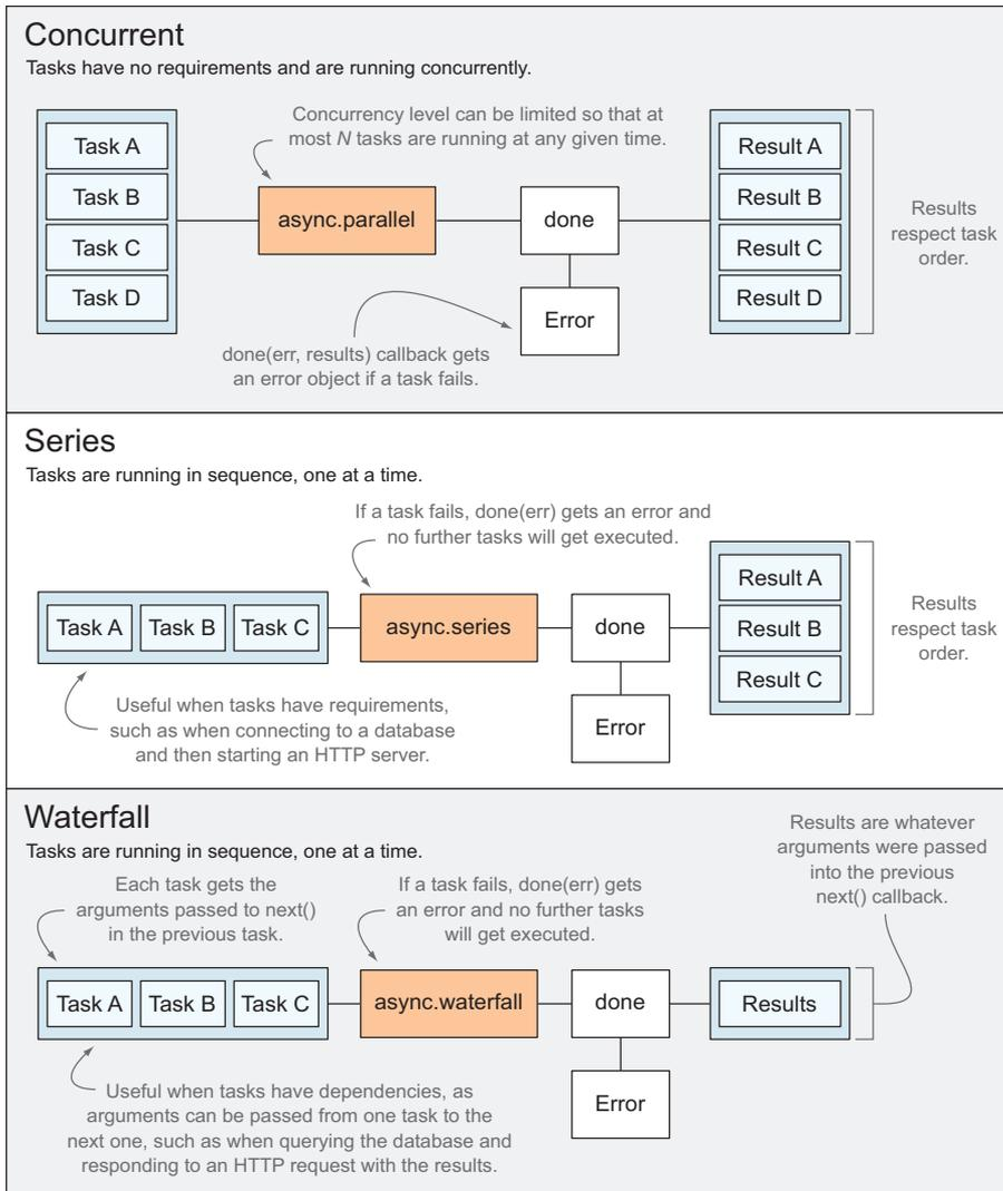
**Figure 6.3** Comparison of parallel, series, and waterfall in the `async` library.
