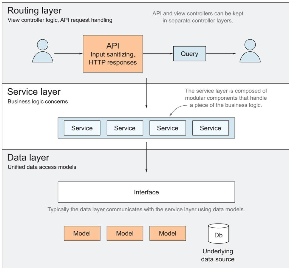
**Figure 9.1** Overview of a three-tiered service architecture
