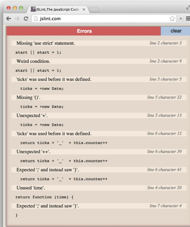
**Figure 1.5** Lint errors found in a code snippet.
