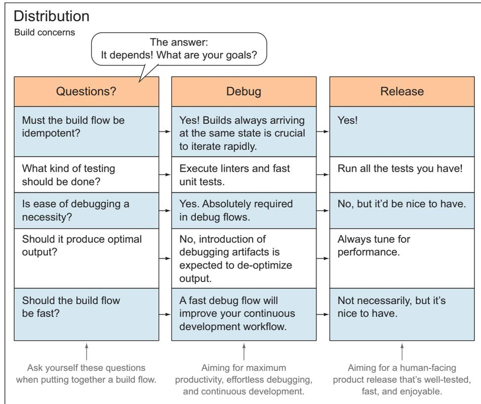
**Figure 3.1** Build distributions and how they define your build flow to fulfill specific goals
