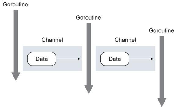
**Figure 1.3** Using channels to safely pass data between goroutines
