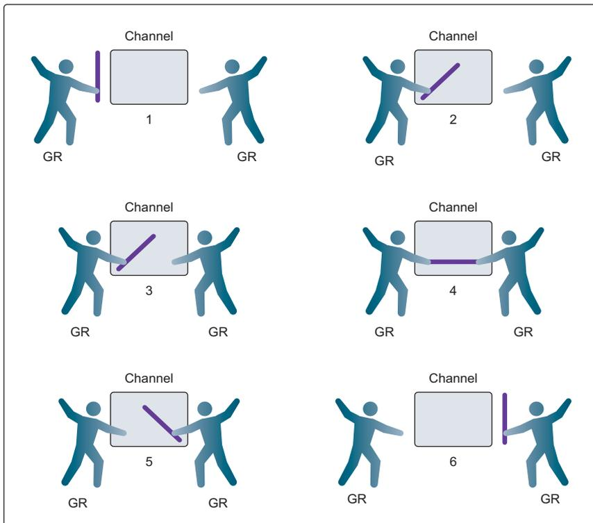
Figure 6.6 Synchronization between goroutines using an unbuffered channel
