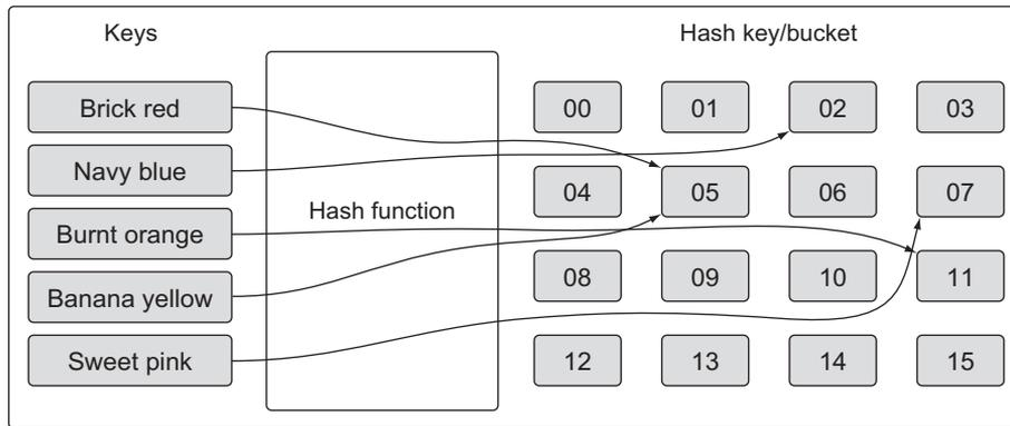
Figure 4.25 Simple view of how hash functions work
