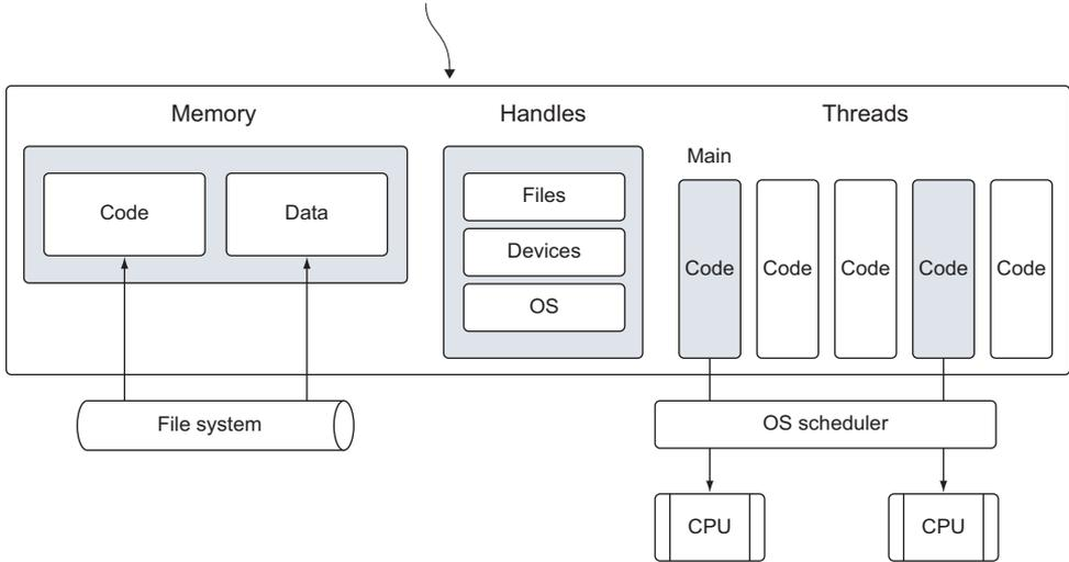
Figure 6.1 A simple view of a process and its threads for a running application
