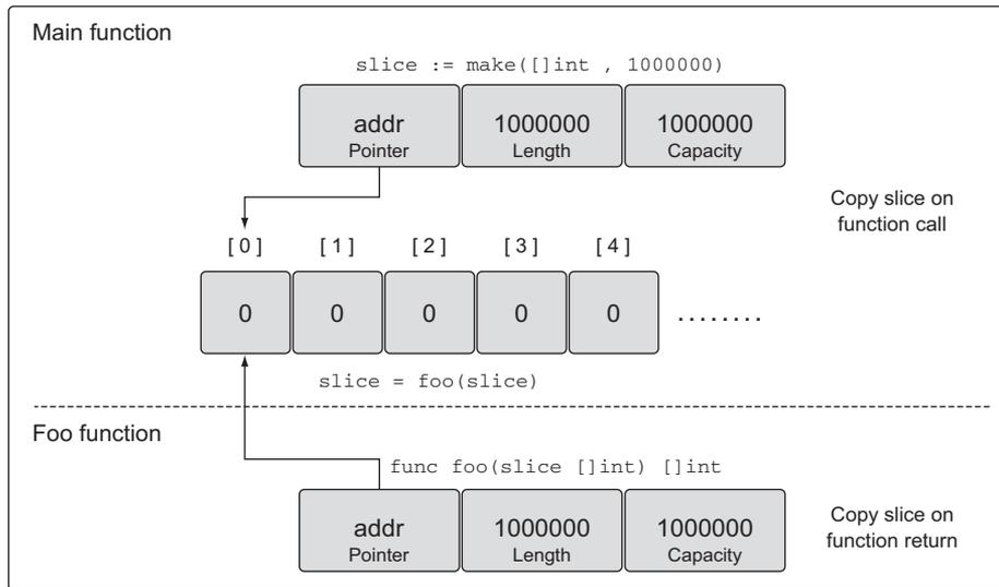
Figure 4.22 Both slices pointing to the underlying array after the function call
