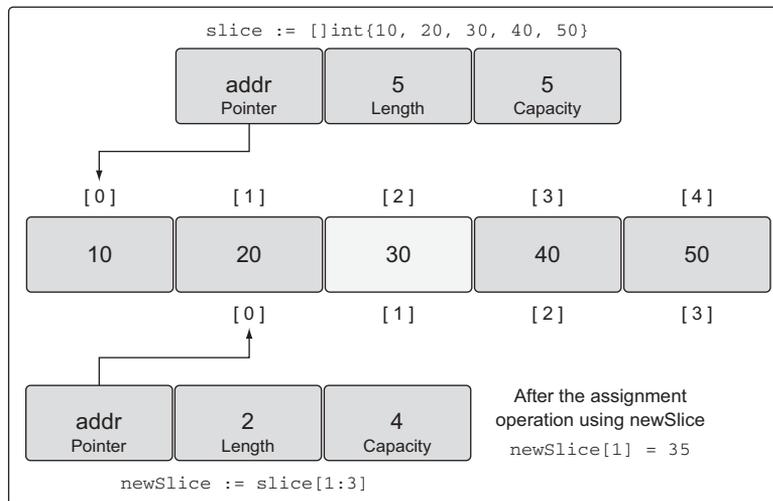
Figure 4.13 The underlying array after the assignment operation
