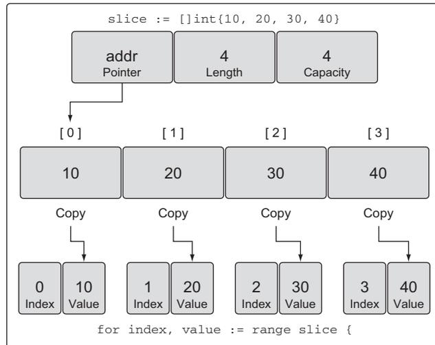
**Figure 4.19** Using `range` to iterate over a slice creates a copy of each element.
