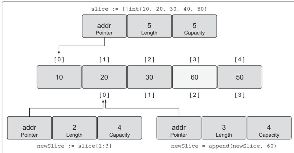
**Figure 4.14** The underlying array after the append operation
