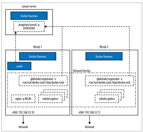
Figure 10-5. Dynamic load balancing of a Galera cluster
