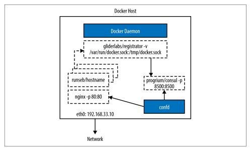
Figure 10-3. Dynamic load-balancing schematic
