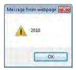
FIGURE 4-6 The output from the getYear() method n nternet Exp orer 8 shows the fu year.
