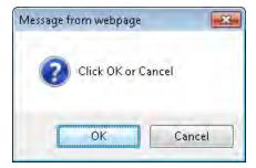
FIGURE 7-6 The confirm() JavaScr pt funct on prov des a d a og box for confirm ng user act ons.
