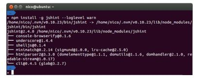
Figure 1.7 Installing jshint through npm
