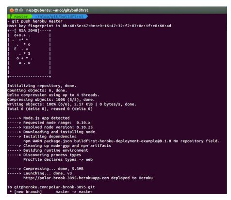
Figure 4.4 Deploying to Heroku—as simple as git push
