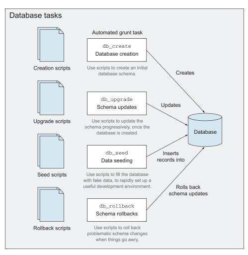
Figure 2.7 Interaction of proposed tasks with a database instance
