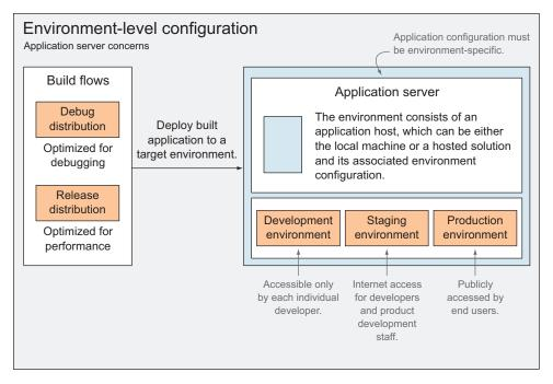
Figure 3.2 Environment-level configuration—environments, configuration, and distributions, coming together in an application. Environment configuration consists of secret credentials and any other configuration that might change across environments.
