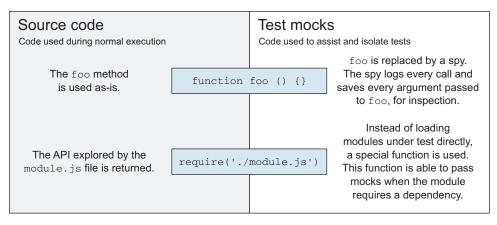
Figure 8.2 Using source code as-is versus using mocks when testing
