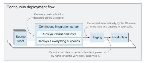
Figure 4.6 Proposed continuous deployment flow
