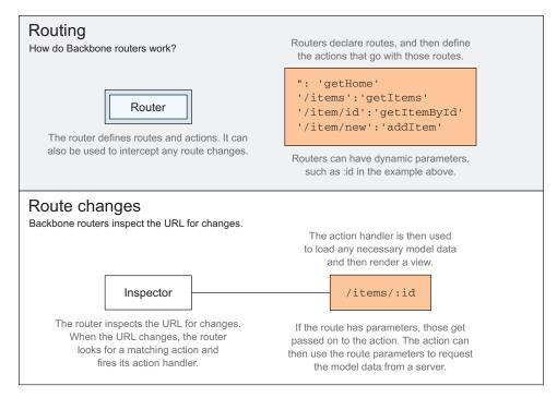
Figure 7.4 Routing in Backbone and the route inspector
