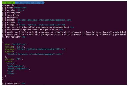
Figure 5.5 Using bower init to create a bower.json manifest file
