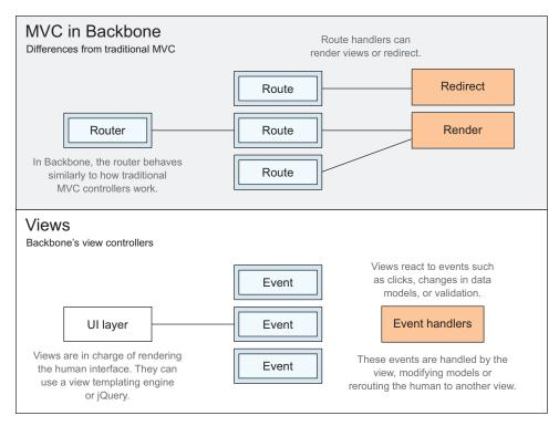
Figure 7.3 Backbone deals with the human-facing aspects of MVC: event handling, validation, and UI rendering.
