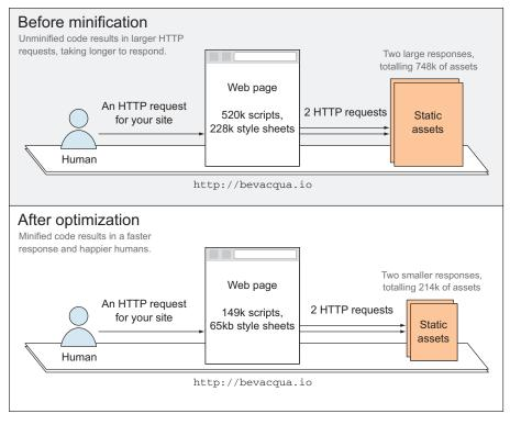
Figure 2.6 Reducing HTTP response length with asset minification
