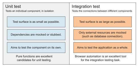
Figure 8.1 Differences between unit and integration testing strategies. Note that a combination of the two should be used. Unit tests and integration tests are not exclusive. Pure functions are discussed in section 8.1.15.
