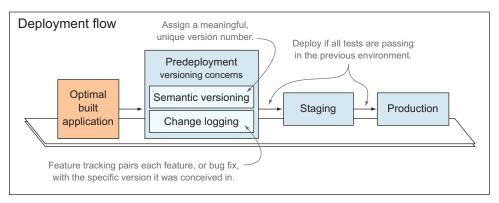
Figure 4.2 Versioning before a deployment and progressive deployment rollout. Testing by QA team in staging ensures robustness before deployment to production.
