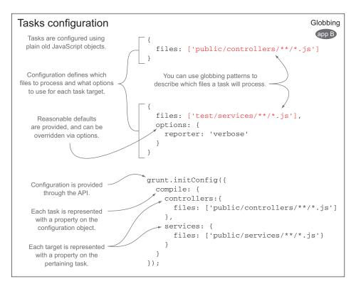
Figure 2.2 Grunt task configuration in code explained. Each task and task target is configured individually.
