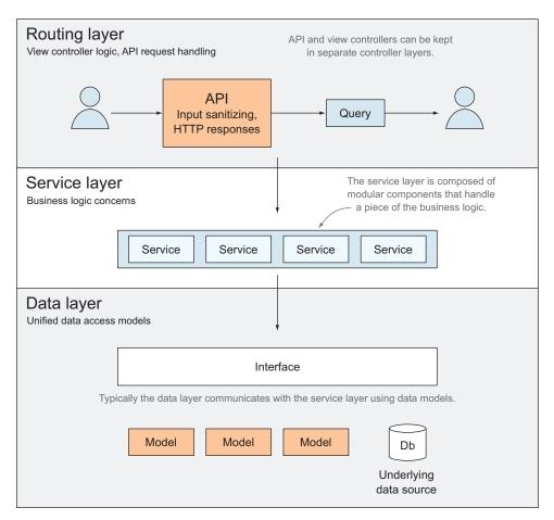
Figure 9.1 Overview of a three-tiered service architecture
