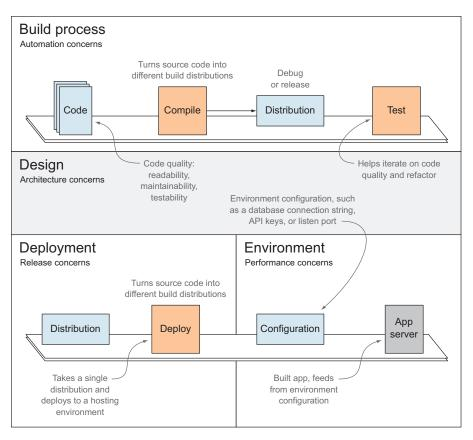
Figure 1.1 High-level view of the four areas of focus in Build First: Build process, Design, Deployment, and Environment
