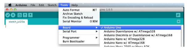
Figure 6-3. Arduino IDE board selection menu
