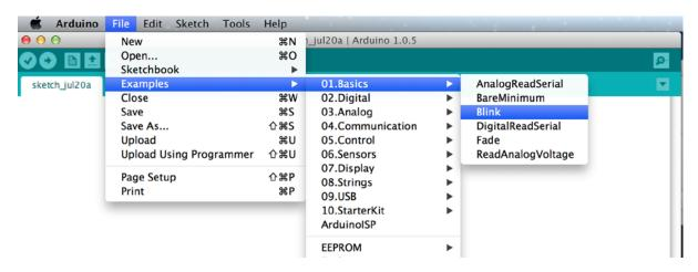
Figure 6-4. Arduino IDE example selection menu
