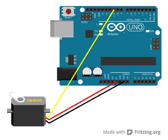
Figure 6-7. Wiring diagram for servo example
