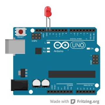
Figure 6-2. Board layout for the blink example
