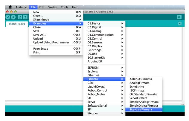
Figure 6-6. Arduino IDE Firmata selection menu
