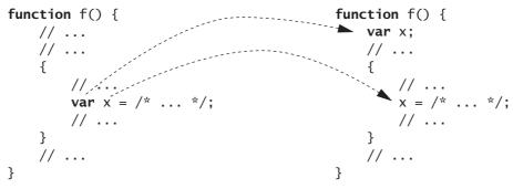
Figure 2.2 Variable hoisting
