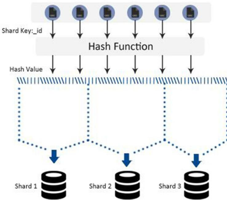
**Figure 7-18.** Hash-based partitioning
