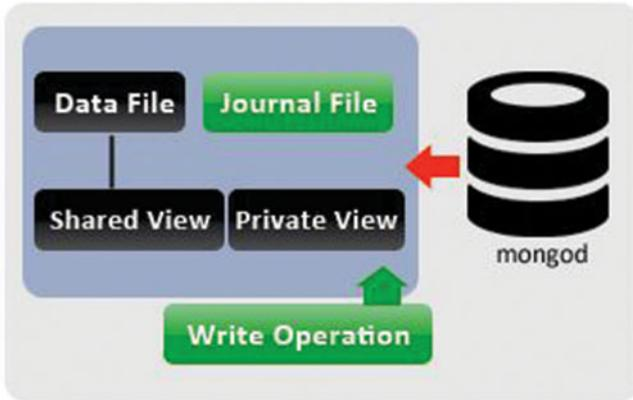
**Figure 8-18.** *Initiated write operation*
