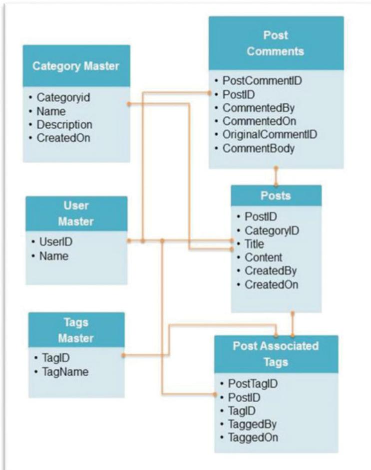
**Figure 6-3.** RDBMS diagram
