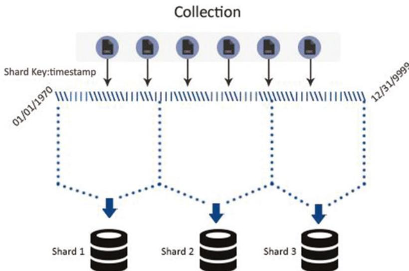
**Figure 7-17.** Range-based partitioning
