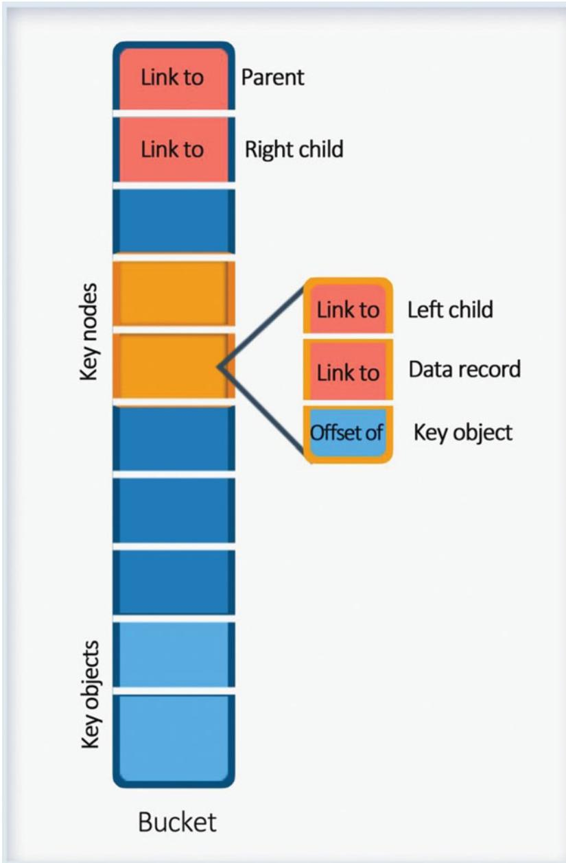
**Figure 8-10.** BTree bucket data structure
