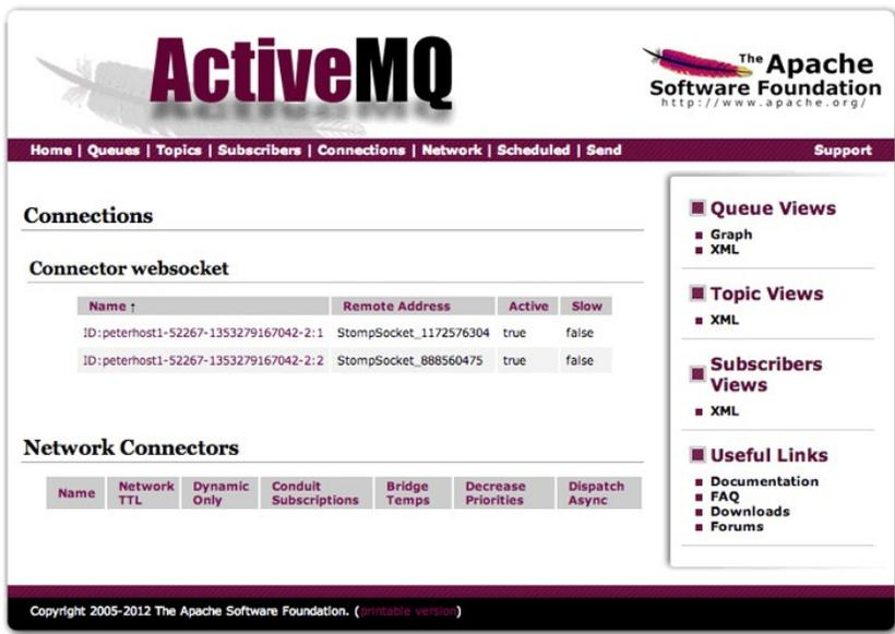
Figure 5-14. Active ActiveMQ connections created through the WebSocket Connector
