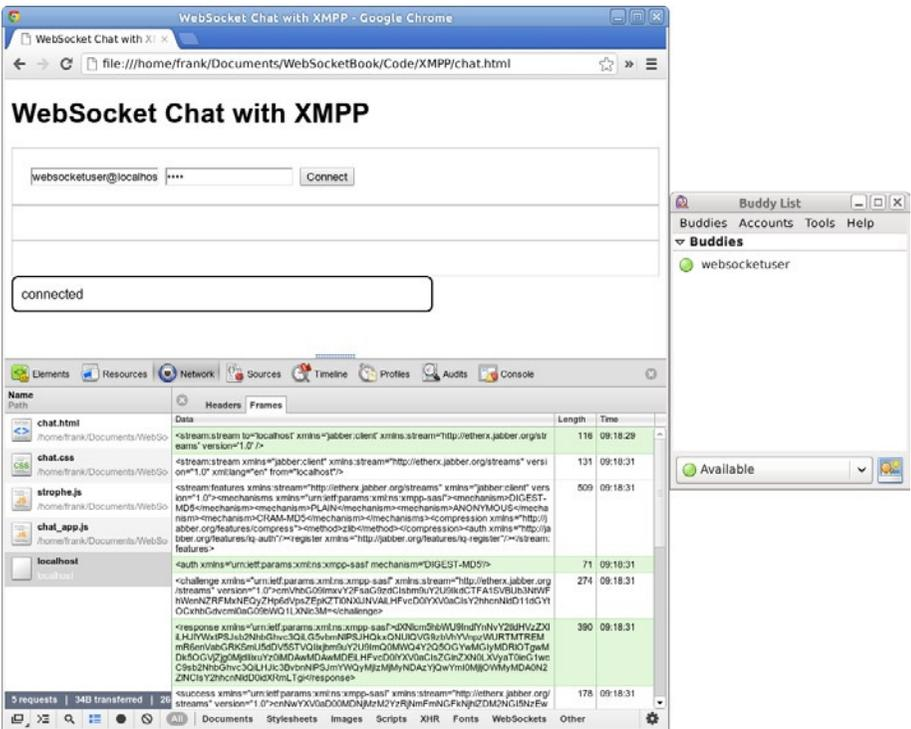
**Figure 4-7.** Logging in from `chat.html` and appearing online in Pidgin. Each WebSocket message displayed in the developer tools contains an XMPP stanza
