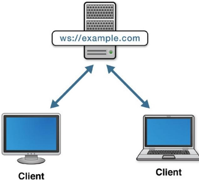
**Figure 3-3.** *WebSocket clients connected to a server*
