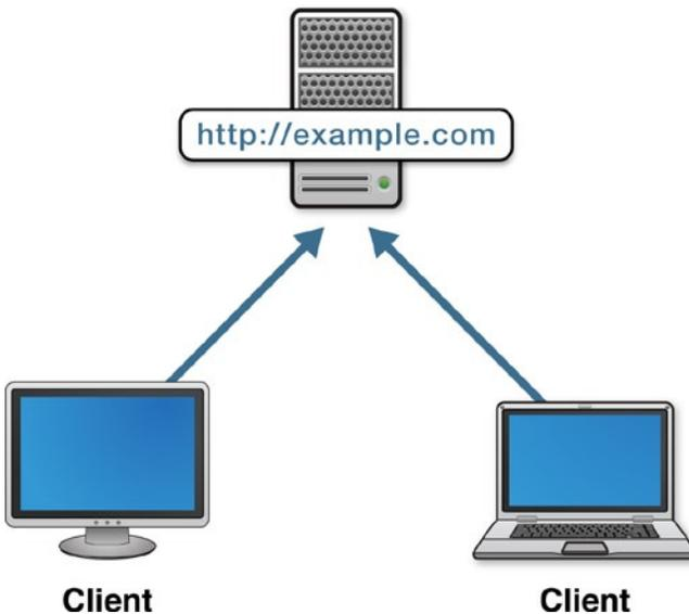
**Figure 3-2.** HTTP clients connected to a Web server
