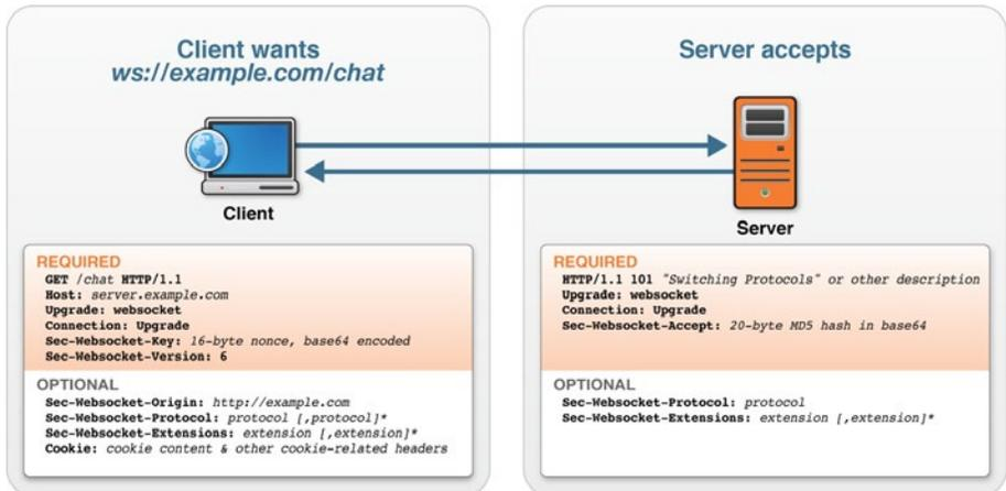
**Figure 3-6.** Example of a WebSocket opening handshake
