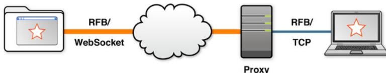
**Figure 6-2.** Connecting with RFB over WebSocket
