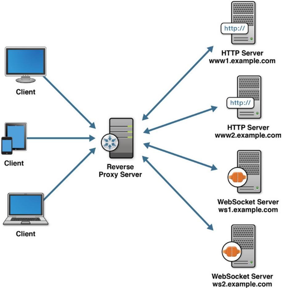
**Figure 8-2.** Reverse proxy server as a load balancer
