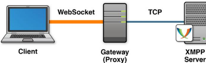
**Figure 4-4.** Connecting to an XMPP server through a WebSocket proxy
